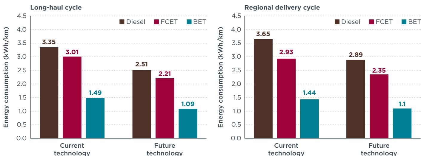
**Figure 15.** Tank-to-wheel electricity equivalent energy consumption of diesel, battery-electric, and fuel cell electric trucks over the long-haul cycle (payload of 19,300 kg and 500 km driving range) and regional delivery cycle (payload of 12,900 kg and 300 km driving range) for current and future vehicle technologies.
