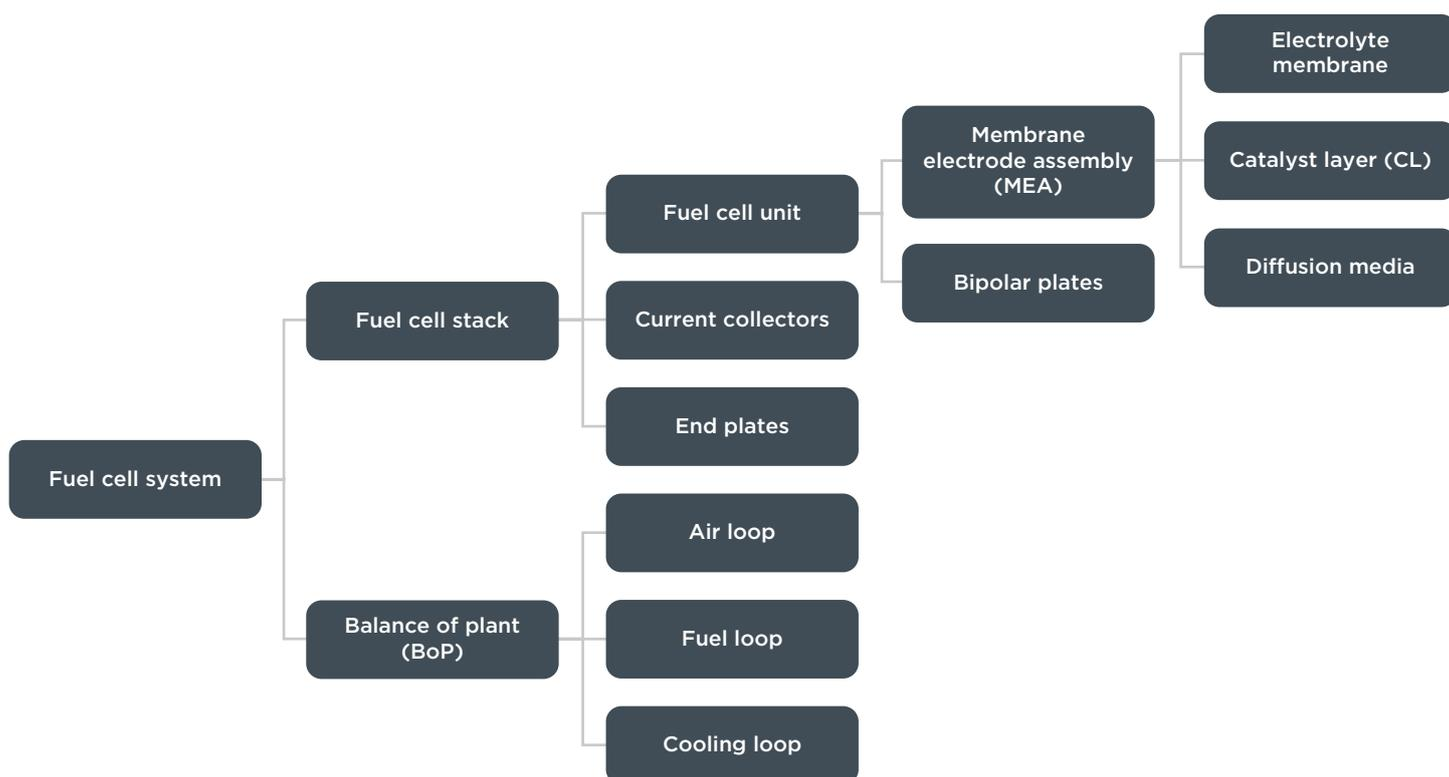
**Figure 2.** Fuel cell system components
