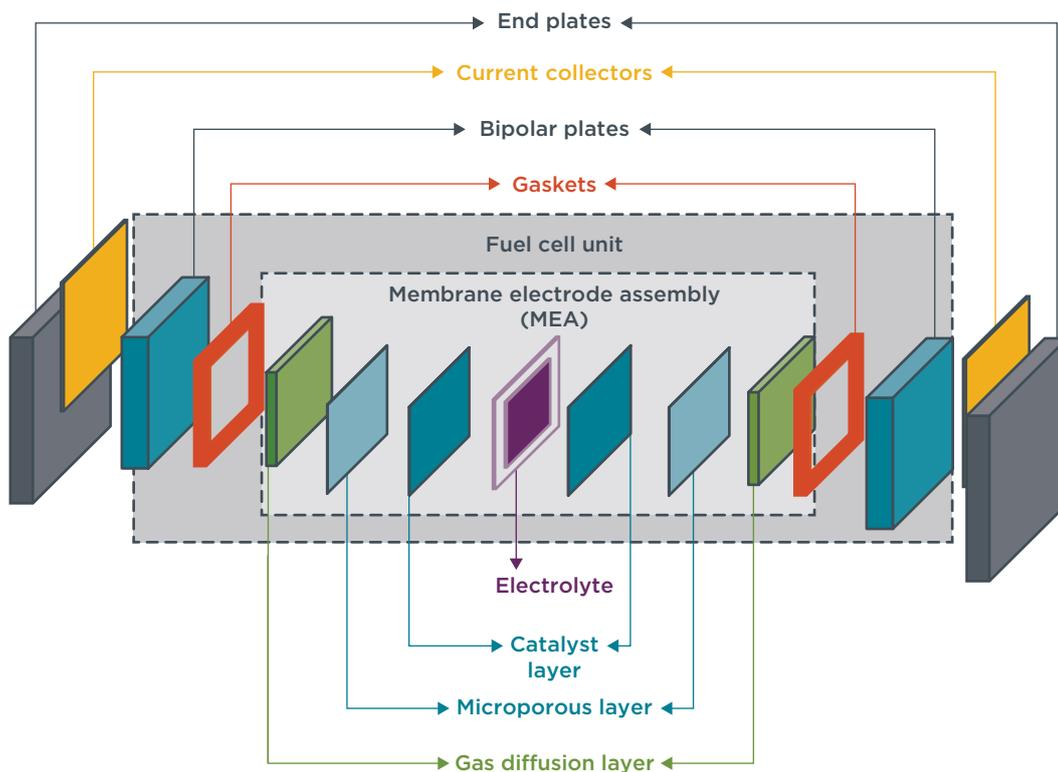
**Figure 3.** Schematic of a fuel cell stack
