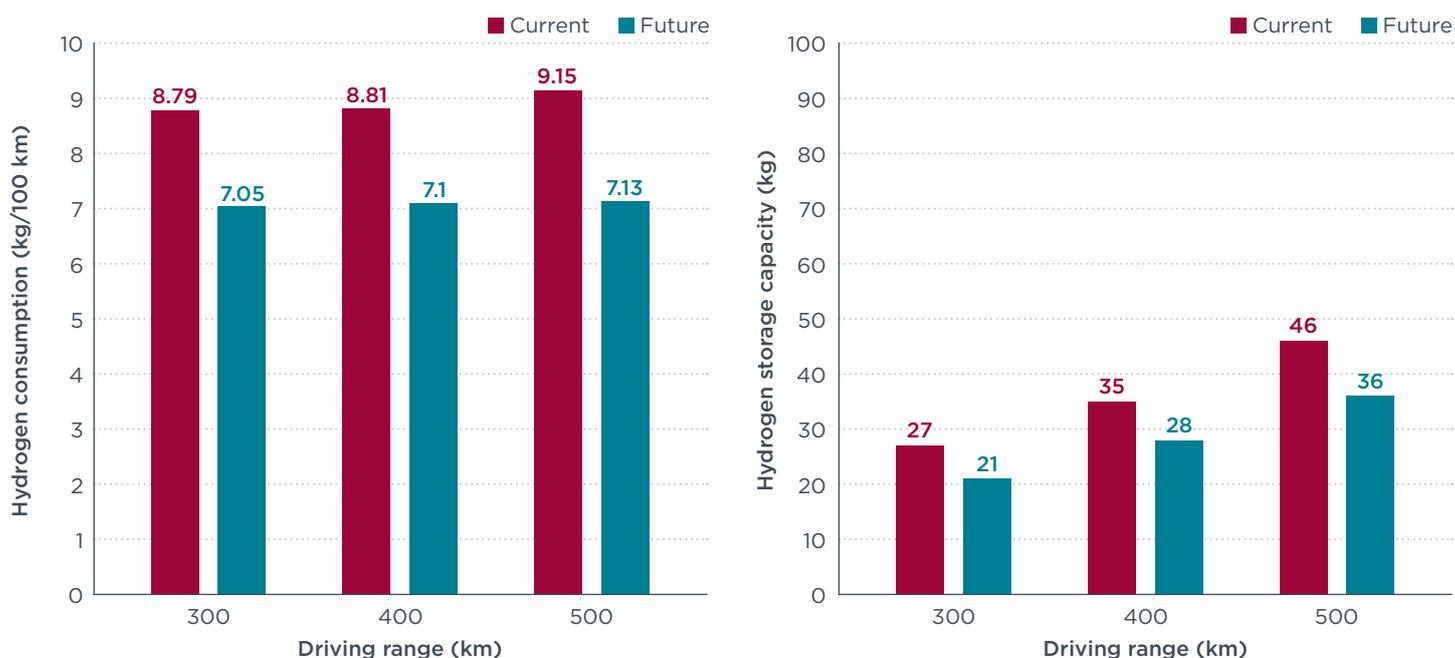
**Figure 11.** Fuel cell electric truck hydrogen fuel consumption (left) and required hydrogen tank size (right) for different driving ranges simulated over the regional delivery drive cycle at a reference payload of 12,900 kg and 15°C ambient temperature for current and future vehicle technologies.
