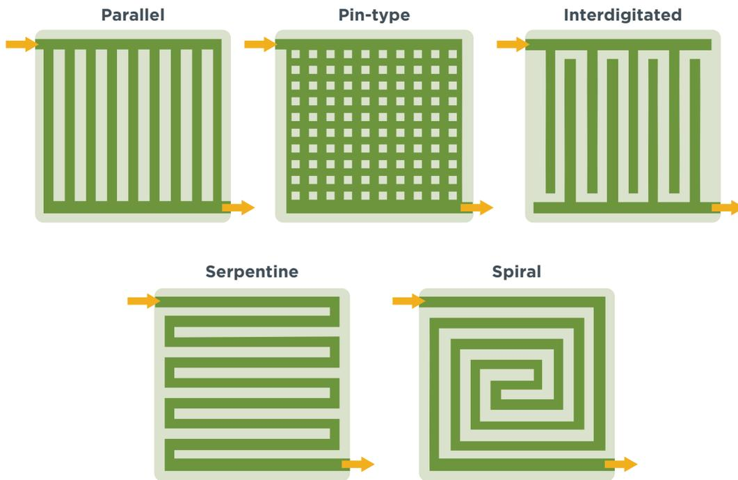
**Figure 5.** Main flow field designs for bipolar plates
