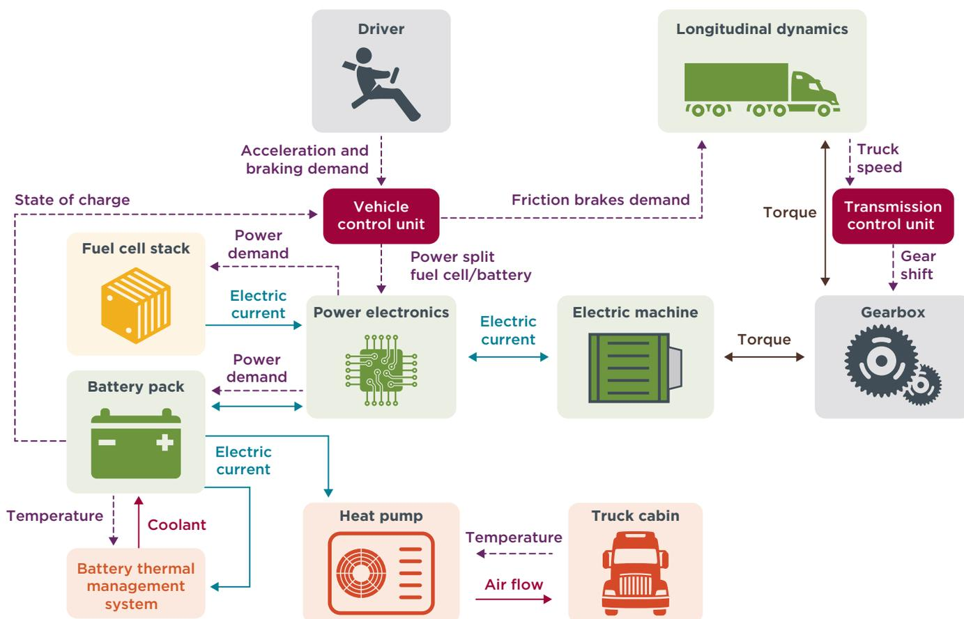
**Figure 7.** Schematic of the truck energy consumption model
