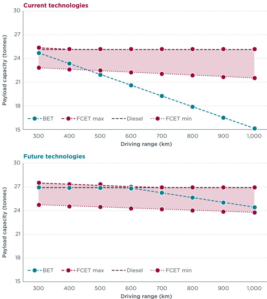
**Figure 17.** Payload capacity of battery-electric, fuel cell electric and diesel trucks at different driving ranges under current and future vehicle technologies. Simulated over the long-haul cycle at a reference payload of 19,300 kg and 15°C ambient temperature.
