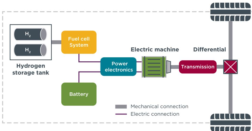
**Figure 1.** Fuel cell electric vehicle powertrain architecture
