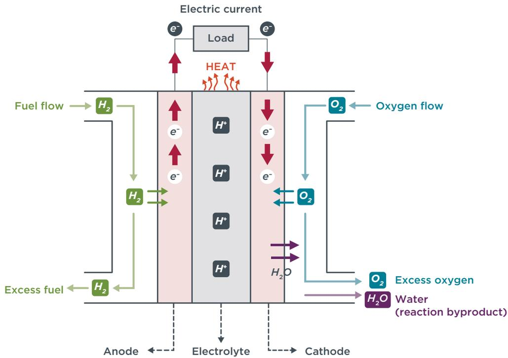
**Figure 4.** Working principle of a fuel cell unit
