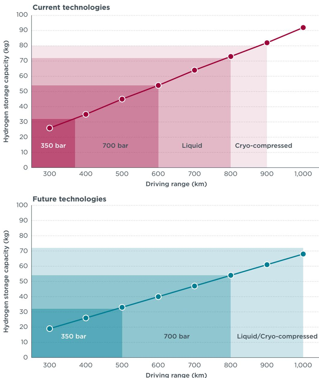
**Figure 14.** Maximum achievable FCET driving range for different hydrogen storage technologies for current and future vehicle technologies considering onboard volume constraints for hydrogen storage.
