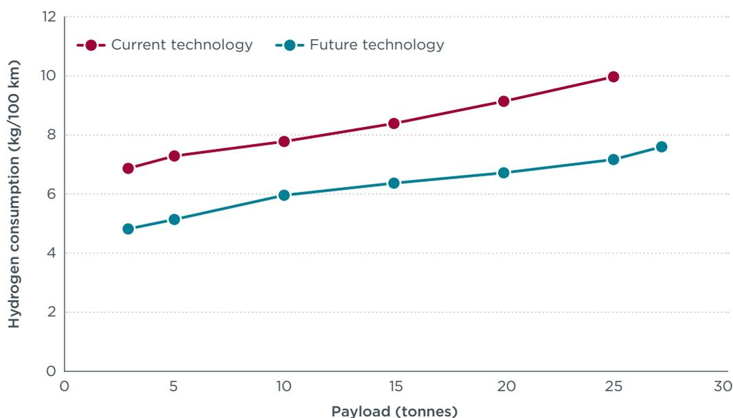
**Figure 12.** Fuel cell electric truck hydrogen fuel consumption at different payloads simulated over the long-haul cycle for current and future vehicle technologies based on a 15°C ambient temperature (hydrogen tank design of 500 km).
